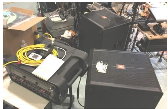
Preparing to test a pair of commercial 18in subwoofers with very good frequency response and distortion data, below. When operated below their design maxima, most SWs exhibit distortion falling much faster than SPL. [Filmmaker Technology]
