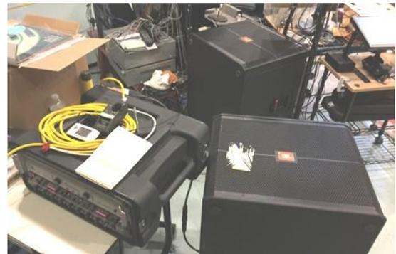
Preparing to test a pair of commercial 18in subwoofers with very good frequency response and distortion data, below. Operated below their design maxima, SWs exhibit distortion falling much faster than SPL. [photo Filmmaker Technology]
