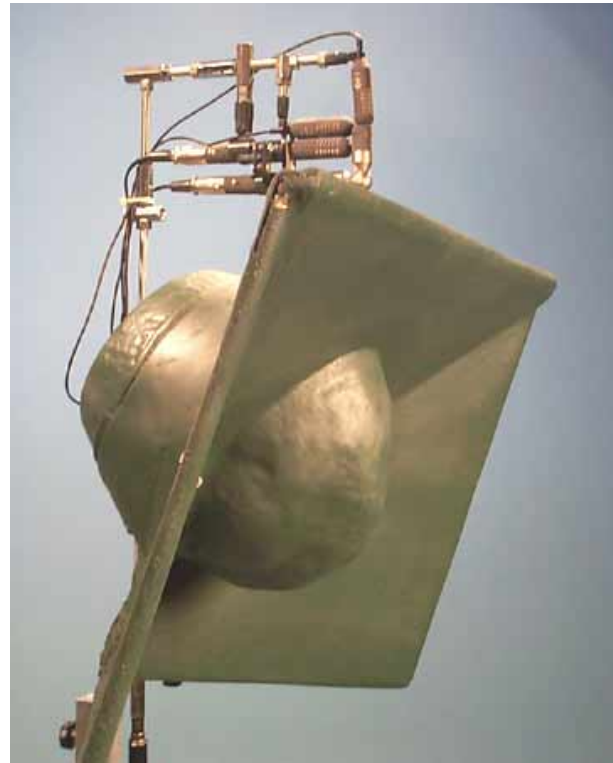
Fig.9 - New design of the PanAmbiophone. Two pairs of small pressure microphone elements are coincident at “ear” positions. A discrete soundfield array is mounted atop – a total of eight recording channels for PerAmbio 3D (with height).
