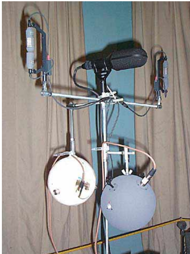
Fig.5 - Original PanAmbiophone using two spheres (barrier removed), OCT, and Soundfield microphones for comparison.
