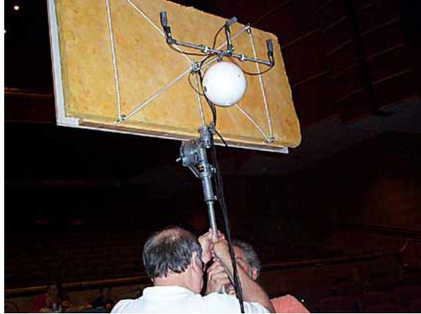
Fig.4 – The first PanAmbiophone with OCT for comparison experiment. Barrier hides second sphere for rear stage.
