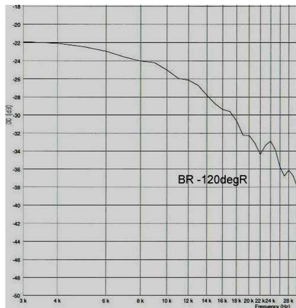
Fig.18 - Unequalized frequency response 3kHz~30kHz of the PanAmbiophone back channels for a source positioned \pm 120^\circ (ipsilateral).
